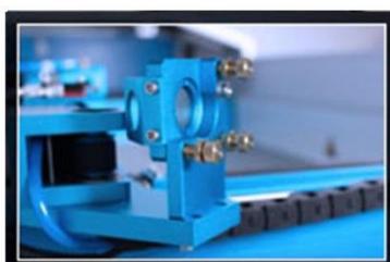
Mirror mount Easily re-adjusting 3D mirror mounts.
