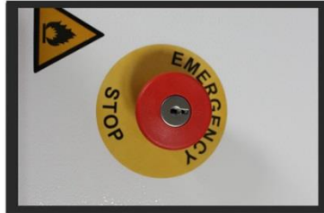
Emergency stop Turn off the machine immediately when there is an accident.
