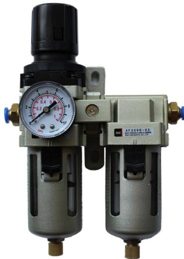
When we use the High pressure air compressor for blowing air, it will absorb much moisture with air at the same time. If we just let the moisture go, they will gather on the focus lens, and when the laser working, the water (moisture) will heat that may lead the lens break. Thus we need a water separator for help, it can stop moisture reaching lens. Water separator was installed between the air compressor and laser head.
