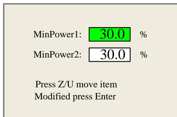
When “Z/U” key is pushed, the green block can move up and down to denote the changing item, then “Y+/-” keys and “X+/-” keys can be used to change the value.
