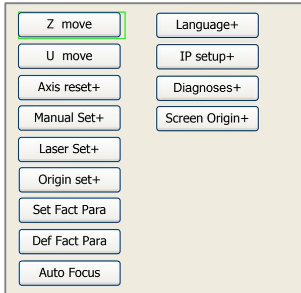
Press up and down arrow keys to move the green block to the anticipated item, and then push the “Enter” key to display the sub menu.
