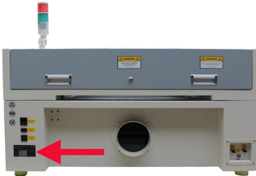
It is recommended to enter data such as serial number and year of manufacture into the manufacturer's label below so that you always have this data handy if you have problems with your device or require spare parts.
