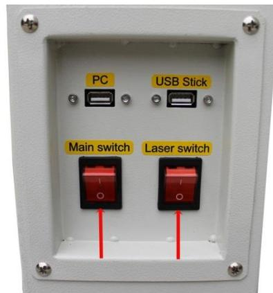
If all covers are closed, immediately after being switched on, the device starts the referencing process. When the referencing process is completed correctly, an acoustic signal sounds and the device is ready for operation. The operation panel will display the home screen when the laser is completed resets.
