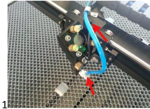
Remove the air pipe and the autofocus
