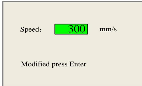
Push the “X+/-” Keys to move the cursor in the numeral area, and push the “Y+/-” keys to change the value, then push the “Enter” key to save the change, push the “Esc” key to invalidate the change.
