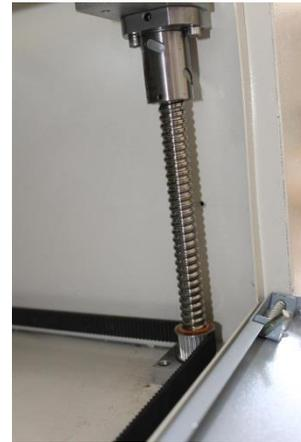
It is suggested to add lubricant oil (or Rust Preventative Grease) to the rails/screws at least every two weeks.
