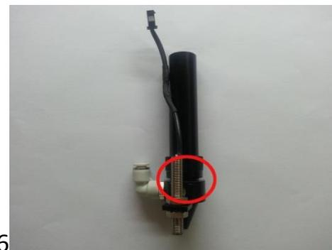
Fixed back the focus lens, and please be careful not to scratch the lens, then merge both parts together
