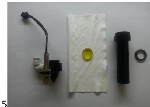
Installation and please concave downward (convex side of the lens is facing upwards)
