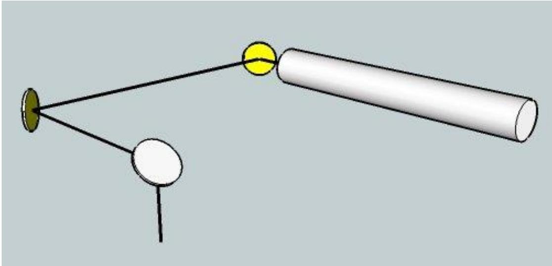
After being used for a long time, the beam path might be deflective. This will reduce the efficiency of the laser beam or even cause no laser beam. At this moment, you will need to re-adjust the beam path again.
