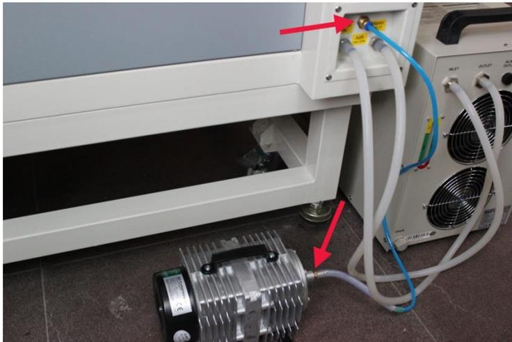
The input voltage must correspond (AC 220 V/50 Hz or AC 110 V/60 Hz) – see information label beside the connection socket.
