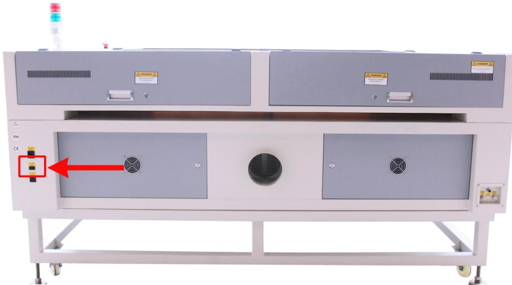
The input voltage must correspond (AC 220 V/50 Hz or AC 110 V/60 Hz) – see information label beside the connection socket.
