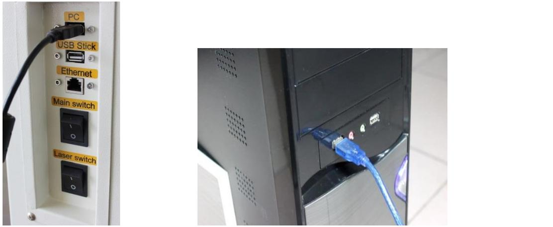
Connecting the Computer and the machine by using the Ethernet cable. Like below:
