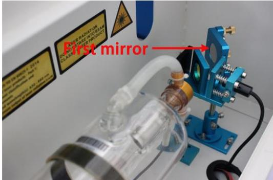
The mirrors are easily get dirty. And this will reduce the efficiency of the laser beam. Meanwhile, laser energy absorbed by the mirror may cause heat and destroy the mirrors too. For the first mirror, you can clean them directly.
