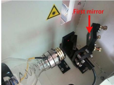
The mirrors are easily get dirty. And this will reduce the efficiency of the laser beam. Meanwhile, laser energy absorbed by the mirror may cause heat and destroy the mirrors too. For the first mirror, you can clean them directly.
