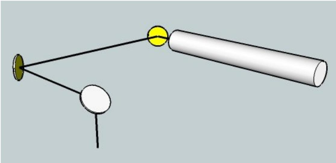
After being used for a long time, the beam path might be deflective. This will reduce the efficiency of the laser beam or even cause no laser beam. At this moment, you will need to re-adjust the beam path again.
