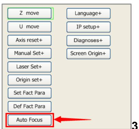
**PS: please do not use "auto focus" function while laser head is HR laser head or 4" laser head.**
